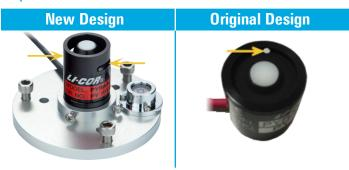
New sensors provide improved water shedding and drainage than the original design.
